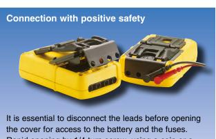
Rapid opening by 1/4 turn screw, using a coin or a screwdriver.
