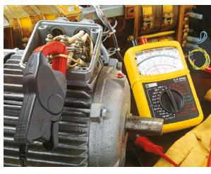
▲ Direct reading of the motor current with the C.A 5005 and its MN 89 miniclamp, supplied as standard. The A AC ranges are marked by the ♠ symbol and also the readout scale.
