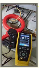
Measurement with leakage current clamp and recording of the fault.
