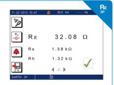
As it is performed with the power off, this is the only earth measurement possible on an installation which has not yet been hooked up to the electrical power distribution network or which is no longer connected to it. Once the cables have been connected, implementation is particularly simple.
