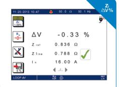
conductor is sufficient for the installation. The result of this  $\Delta V$  measurement is displayed in %; if the value is greater than 5 % or a programmed value, the sizes of the cables for the installation must be recalculated.
