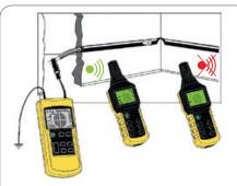
Detection of the pinched or obstructed part in a non-metallic pipe
