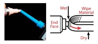
Wet the CCT fabric tip with the MX pen, insert the CCT tip into the connector, and push in the tool 2-3 clicks advancing the fabric from wet-todry, perfectly cleaning the end-face.
