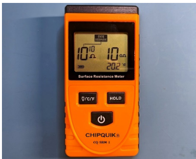
Image 1: Resistance on an ESD work mat (static dissipative)
