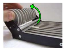
The SMD components tape is shifted forward by winding the foil to the winding wheel. When using short cut tapes (these tapes are mostly wrinkled or damaged- broken), jamming, heavy shift of the tape forward or springing of the components can occur. Therefore it is recommended to straighten the tapes before winding.
