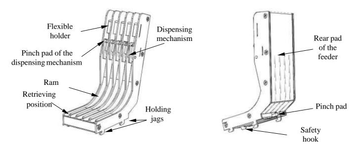
Sliding in the poles with integrated circuits (IC):): Remove the ICF from the assembling desk and put it rear down onto the table. Take out the safety catch from one end of the pole so that the IC does not spill. Slide this end under the flexible holder as far as it goes. Repeat the procedure for the required number of positions.
