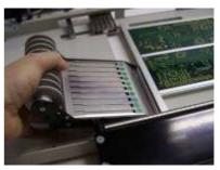
Tilt the left hand support. Grab the feeder from behind and lean it slightly forwards. Plug the feeder into the slot for feeders in such way that the jags on front part of the feeder got under the metal plate of the assembling desk. After the right plugging will the jags fit into the bottom rear sockets, which ensures that the feeder will not accidentally move when on the assembling desk. Take down the left hand support in the end.
