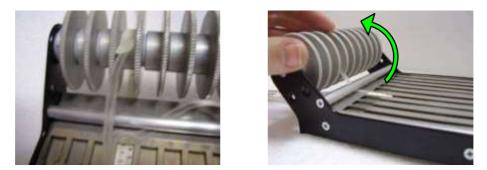
The SMD components tape is shifted forward by winding the foil to the winding wheel. When using short cut tapes (these tapes are mostly wrinkled or damaged- broken), jamming, heavy shift of the tape forward or springing of the components can occur. Therefore it is recommended to straighten the tapes before winding.
