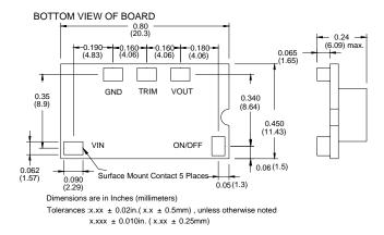
Figure 21 SMT05 Mechanical Outline Diagram
