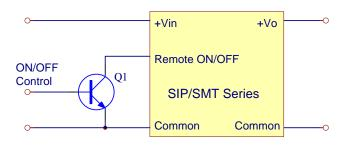
Figure 3. Positive Remote ON/OFF Input Drive Circuit
