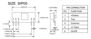
Figure 20 SIP05 Mechanical Outline Diagram
