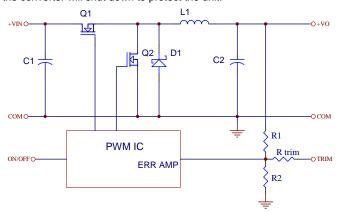
Figure 1. Electrical Block Diagram
