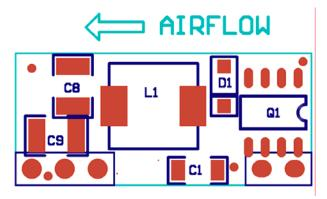
Figure 8. Temperature Measurement Location for SIP
