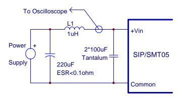
Figure 14. Input Reflected-Ripple Test Setup
