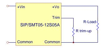
Figure 17. Trim-up Voltage Setup
