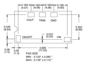
Figure 6. Recommended SMT Footprint (Top View)
