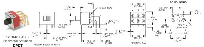
Not available with M1 mounting style, I seal option. Terminal bend radii and lead-in manufacturing option.
