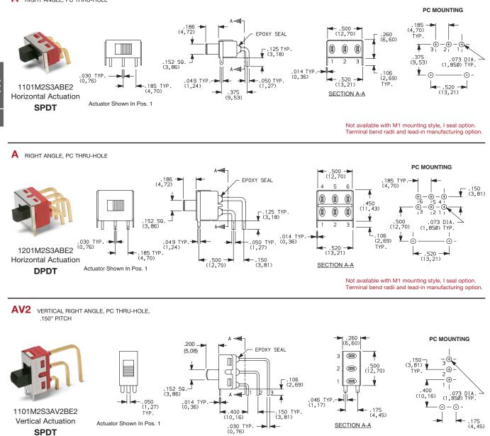
Not available with M1 mounting style, I seal option. Terminal bend radii and lead-in manufacturing option.
