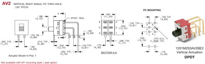
Terminal bend radii and lead-in manufacturing option.
