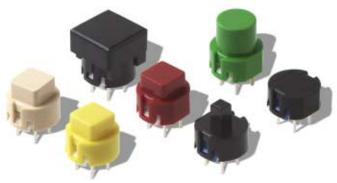
The D6 is a single-pole, momentary action, normally open keyswitch specially designed for digital electronic controls. Its small size enables keyboard design with minimum center spacing of 12.7 mm (0.500).
