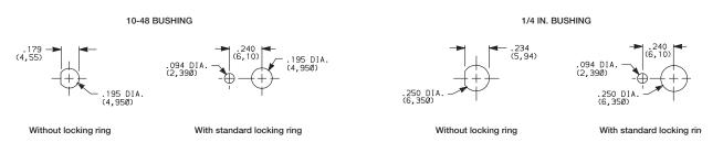
NOTE: One mounting nut, locking ring and lockwasher supplied standard with 10-48 threaded bushings (two nuts with 1/4-40 bushings). Optional mounting nut and locking ring styles and finishes available separately, see section "Technical Data and Additional Hardware".
