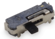
JSM08011SAQNL SPDT Surface Mount Momentary only
