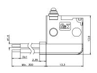
COM: AVSS 0.3 MM<sup>2</sup> BLACK OR EQUIVALENT NO: AVSS 0.3 MM<sup>2</sup> BLUE OR EQUIVALENT NC: AVSS 0.3 MM<sup>2</sup> GRAY OR EQUIVALENT
