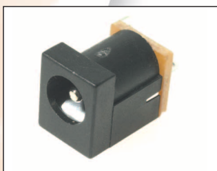
DC-9 PCB mounting pin ring type with switch. Rated 12V / 5A. DC9 with 2.1mm dia. pin. DC9A with 2.5mm dia. pin.
