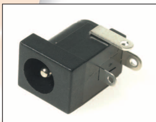
DC-10 PCB mounting pin / ring type with switch. Rated 12V / 5A. DC10A with 2.1mm dia. pin. DC10B with 2.5mm dia. pin.
