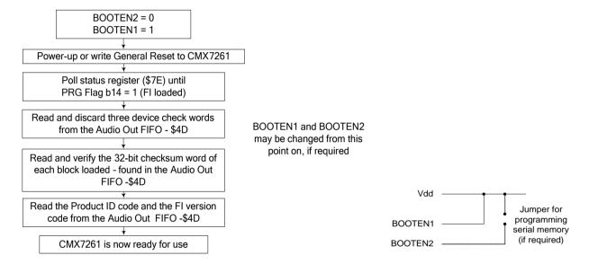
Figure 18 FI Loading from Serial Memory
