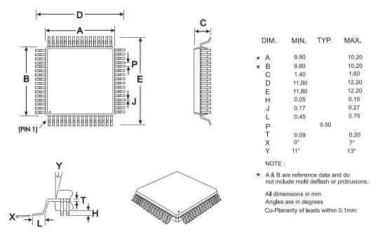
Figure 35 Mechanical Outline of 64-pin LQFP (L9)
