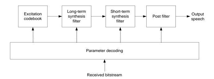
Figure 19 Block Diagram of Conceptual CELP Synthesis Model
