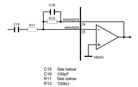
Figure 13 Recommended External Components - Single-Ended Audio Input Interface
