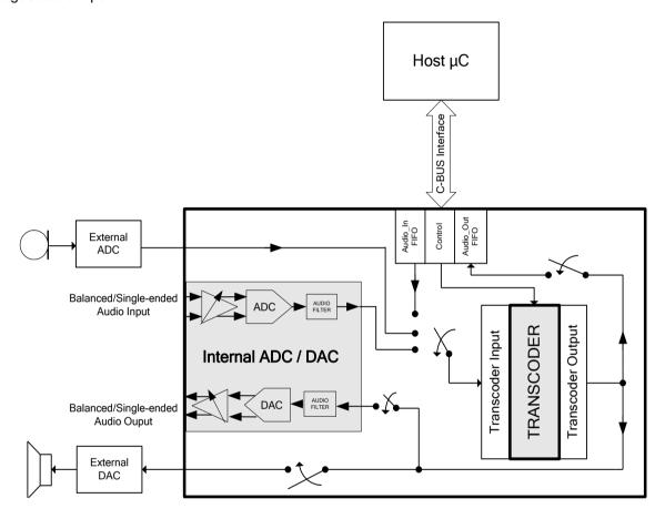
Figure 14 CMX7261 Inputs and Outputs
