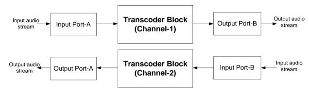
Figure 2 Full Duplex Block Diagram
