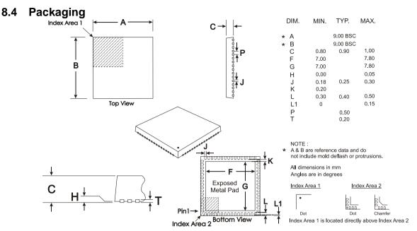
Depending on the method of lead termination at the edge of the package, pull back (L1) may be present.
