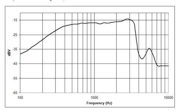
Figure 29 CVSD 16kbps Frequency Response
