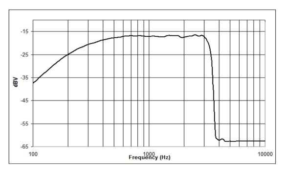
Figure 30 CVSD 32kbps Frequency Response
