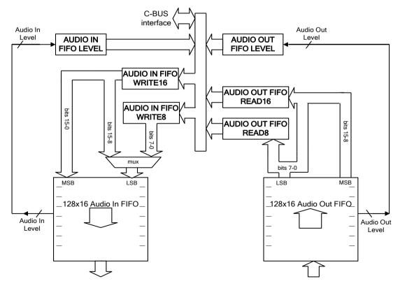
Figure 22 Audio Input and Audio Output FIFOs
