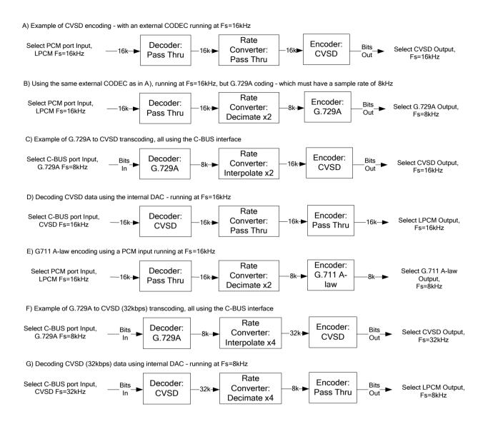
Figure 25 Examples of Sample Rate Conversion
