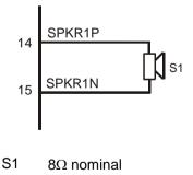
Figure 11 Recommended External Components - Speaker1 Output
