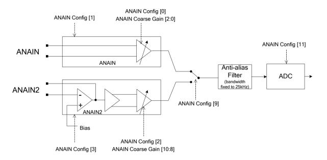
Figure 12 Analogue Audio Input Routing
