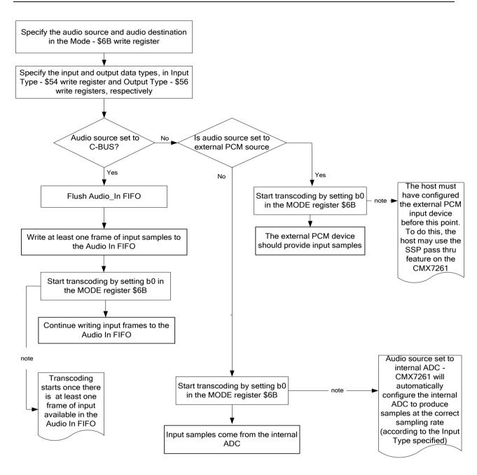
Figure 23 Input Data Transfer into the CMX7261
