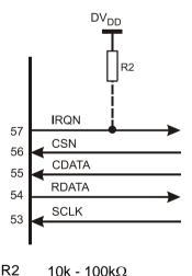
Figure 5 Recommended External Components - C-BUS Interface
