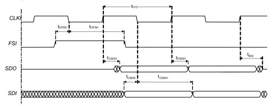
Figure 33 PCM External Clock Timings
