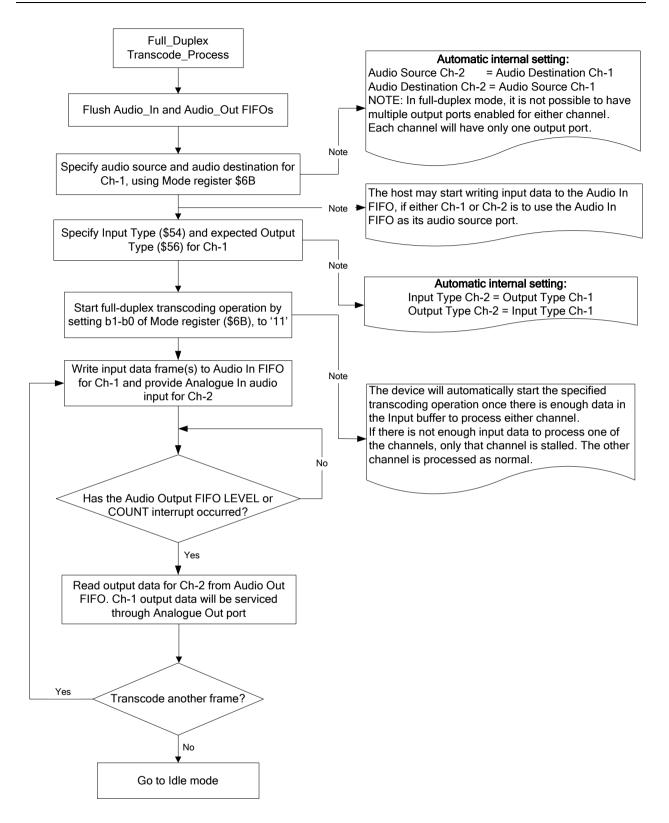
Figure 28 Full duplex Transcoder Operation Flowchart
