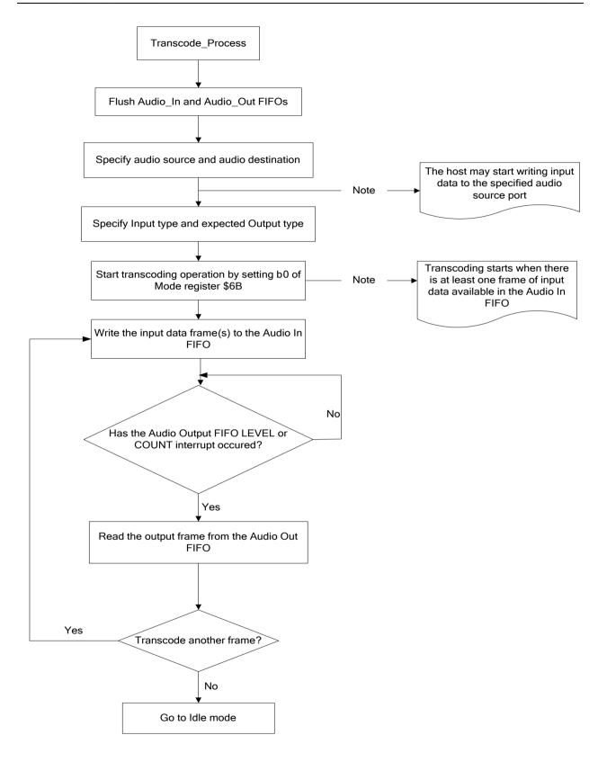
Figure 27 Transcoder Operation Flowchart
