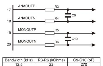
Figure 9 Recommended External Components - ANAOUT/MONOUT Reconstruction Filter
