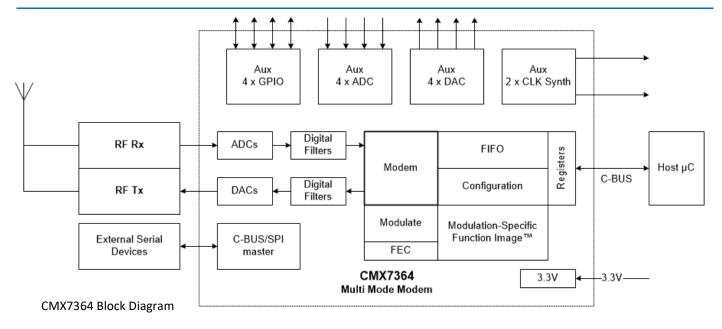
Functionality of the CMX7364 is determined by loading a Function Image™ supplied by CML. The Function Image™ is downloaded on power up and configures the device for the required modulation scheme and associated parameters.
