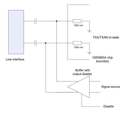
Figure 20 Mixing signals onto the line interface
