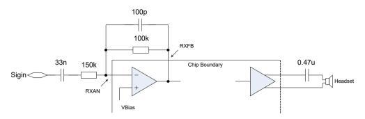
Figure 19 Voice Record and Playback - Test Set-up
