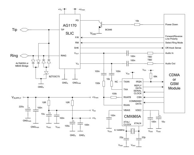
Figure 5 The CMX865A in a Wireless Local Loop Application
