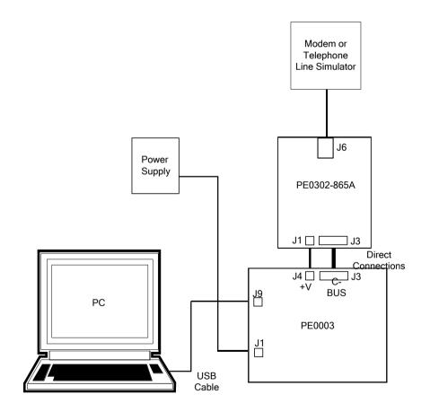
Figure 2 PE0302-865A used with PE0003
