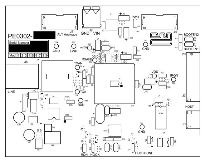
Figure 3 Evaluation Board Layout - Top
