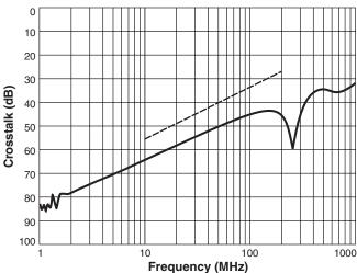
802.3af specification: 45 dB min at 30 MHz 40 dB min at 60 MHz 33 dB min at 100 MHz
