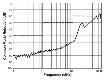
802.3af specification: 50 dB min from 1 MHz to 10 MHz
