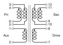
The primary and secondary windings are to be connected in parallel on the PC board.
