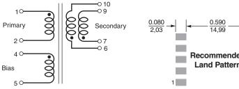
Secondary windings to be connected in parallel on PC board
