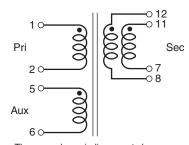
The secondary windings are to be connected in parallel on the PC board.
