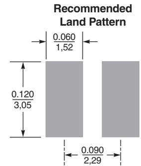
Dimensions are in  $\frac{\text{inches}}{\text{mm}}$
