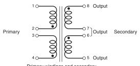
Primary windings and secondary windings to be connected in series on the PC board.
