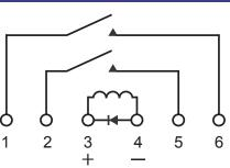
Part Number Example: 3570.1429.xxx 3570.1429.052 = 15 Watt, 2 Form A, 5 volt coil with external shield
