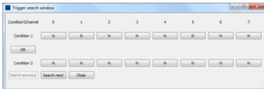
Figure 4-40 Search Signal Pattern
