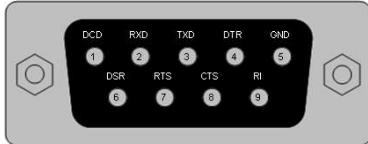
Figure 3-1 RS232 DB9 Pin Out
