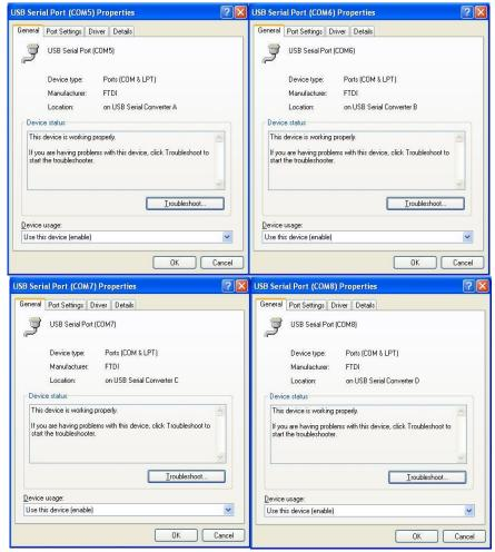
Figure 2.10 - COM Port Assignment and Properties
