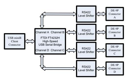
Figure 1.2 USB2-H-6004 Block Diagram
