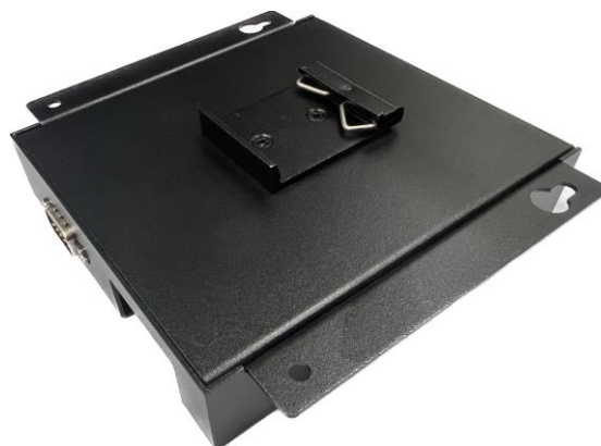
Figure 2-2 - USBC-H-422/485-M PRO or -ISO PRO's Mounting
