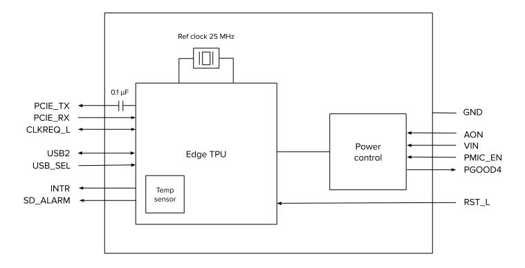
Figure 1. Accelerator Module functional block diagram
