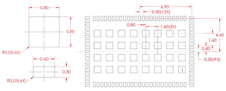
Figure 9. Land pattern dimensions (symmetrical across the X-Y centerlines)
