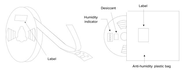
Figure 16. Humidity indicator on plastic package
