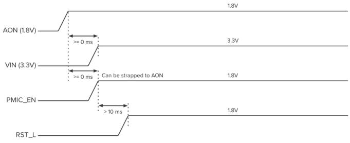
Figure 5. PCIe power-on sequence
