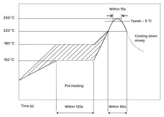
Figure 10. Reflow soldering conditions example
