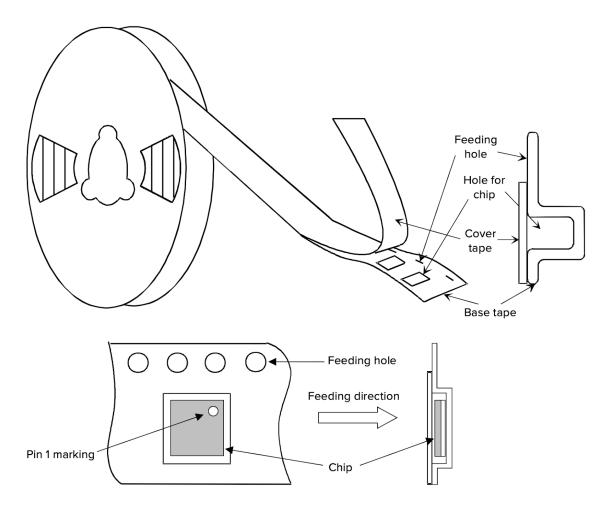
Figure 13. Taping diagram
