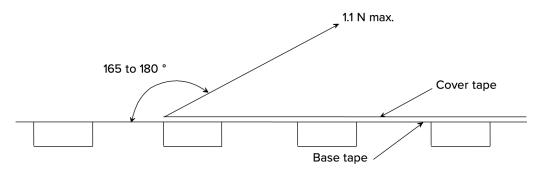
Figure 15. Peeling force diagram
