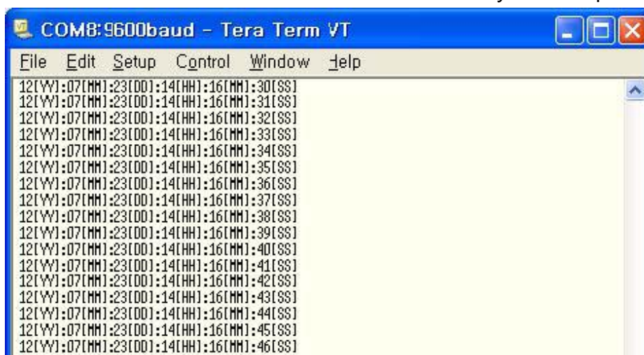
Fig6. CBM1363 RTC Data on Serial Terminal
