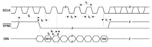
Figure 3. Serial Interface Timing Diagram
