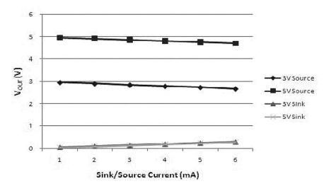
Figure 9. Vout Source and Sink Current Capability
