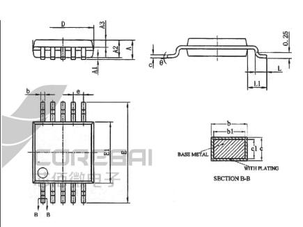
Figure 5 MSOP10L Dimensions shown in millimeters
