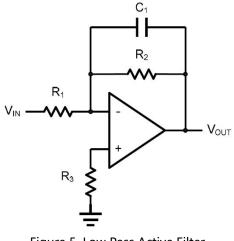
Figure 5. Low Pass Active Filter
