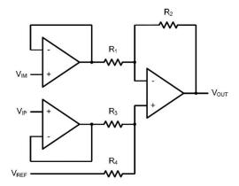
Figure 6. Instrument Amplifier
