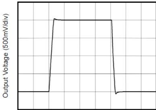
Non-Inverting Large-Signal Step Response
