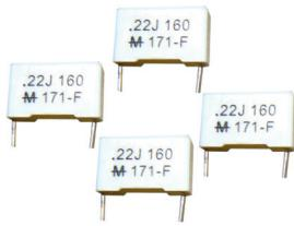
Type 171 radial leaded, box, metallized polypropylene capacitors are available in five pitch sizes and have a flame retardant case and epoxy encapsulant that meets UL94V-0. The Type 171 is an excellent choice for applications requiring low dielectric losses, high insulation resistance in an AC or DC environment. The polypropylene dielectric gives this capacitor excellent pulse rise time (dv/dt) performance.
