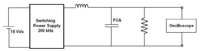
In the above circuit, one 1  $\mu$ F FCA capacitor results in the same ripple reduction performance as a 10  $\mu$ F tantalum capacitor at 200 kHz. With a 1  $\mu$ F tantalum capacitor in the circuit the measured ripple voltage was 70 mVpp, and with a 10  $\mu$ F tantalum or a 1  $\mu$ F FCA capacitor the ripple voltage was 8 mVpp.
