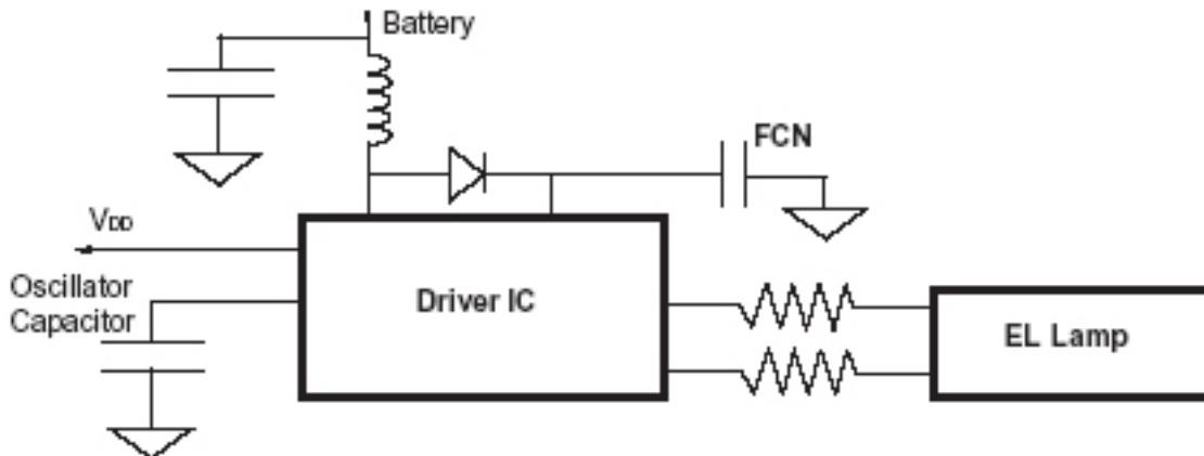
With no piezoelectric effects to deal with, the SMT film capacitor will not create electrical noise in signal circuits or buzzing in power circuits.
