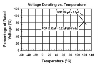
If the temperature on the surface of the capacitor is above 105°C, then the maximum voltage for FCP 50 Vdc ratings from .12 μF to .22μF must be derated linearly from full rated voltage at 105°C to 75% of the rated voltage at 125°C.
