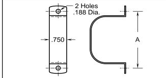
This clamp has a galvanized finish and is designed for use with the flat oval base style AC capacitors, types MPF/MSF. Material thickness is .036"
