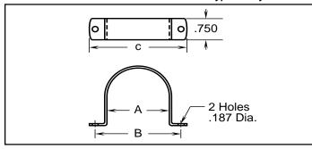
This clamp has a galvanized finish and is designed for use with the round base style motor run capacitor, types MPF. Material thickness is .035"
