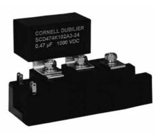
Style SCD offers protection against voltage transients in low to medium current IGBT applications where high dV/dt is encountered. Connect these capacitors from C1 to E2 on a dual IGBT module or from P to N on a six-pack module to eliminate severe voltage transients. Parts ending with Z25 fit IGBTs with 23mm, 25mm and 28mm lead spacing. If you have a preferred lead spacing, please specify.
