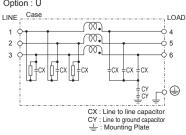
(2) Line to ground capacitor code: 224
