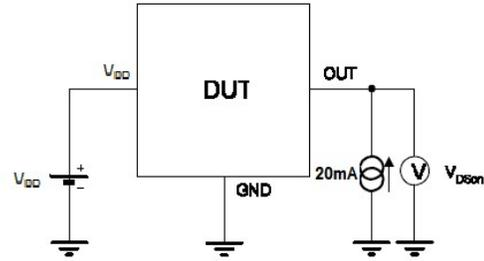
Note 1 - The output saturation voltage  $V_{DSon}$  is measured at  $V_{DD}=3.3V$  and  $V_{DD}=20V$
