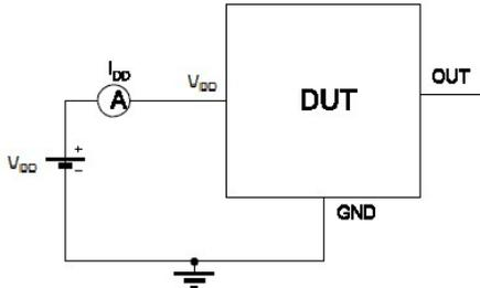
Note 1 - The supply current  $I_{DD}$  represents the static supply current. OUT is left open during measurement
