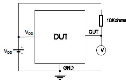
Note 1 -  $B_{OP}$  is determined by putting the device under magnetic field swept from  $B_{RPmin}$  up to  $B_{OPmax}$  until the output is switched on.
