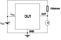
Note 1 - BoP is determined by putting the device under magnetic field swept from BRPmin up to BOPmax until the output is switched on. Note 2 - BRP is determined by putting the device under magnetic field swept from BOPmax down to BRPmin until the output is switched off.
