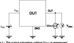
Note 1 - The output saturation voltage  $V_{DSon}$  is measured at  $V_{DD}{=}3.3\,V$  and  $V_{DD}{=}20V$
