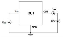
Note 1 - The device is put under magnetci field with B<BRP
