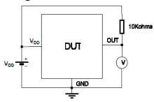
Note 1 - Bop is determined by putting the device under magnetic field swept from BRPmin up to BoPmax until the output is switched on.
