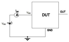
Note 1 - The supply current IDD represents the static supply current.
