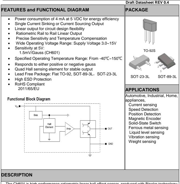
The CH601 is high performance ratiometric linear hall effect sensor, produced with Bipolar technology; it is high performance small versatile linear Hall-effect devices which are operated by the magnetic field from a permanent magnet or an electromagnet. The ratiometric output voltage is set by the supply voltage and varies in proportion to the strength of the magnetic field. The CH601 family has a quiescent output voltage that is 50% of the supply voltage.
