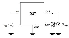
Note 1 - The output saturation voltage VDSon is measuured at VDD=3.8V and VDD=24V
