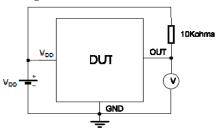
Note 1 - Bop is determined by putting the device under magnetic field swept from BRPmin up to Bopmax until the output is switched on.
