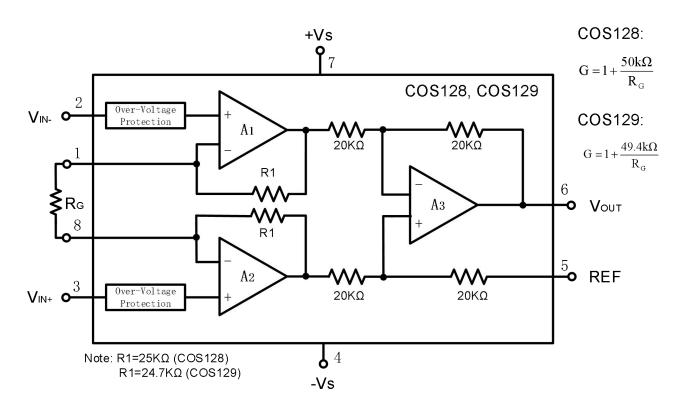
Figure 3.1 Functional Block Diagram
