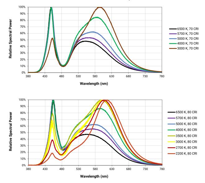
The following graphs are the result of a series of pulsed measurements at 350 mA and T<sub>1</sub> = 85 °C.
